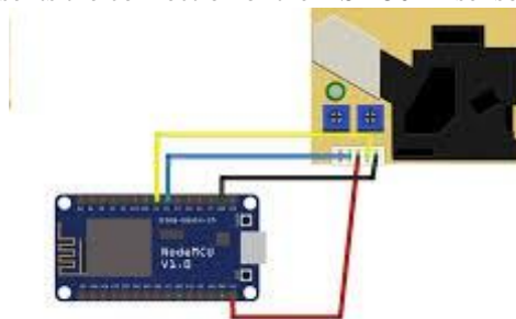
Figure 5: DSM501A Integration with ESP8266
