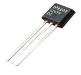
LM35 sensor is used for measurement of body temperature. Sensor is put in contact with body and it senses body temperature. It is calibrated linearly in Celsius. It has low self-heating capability. Also, it doesn't require external calibration.
