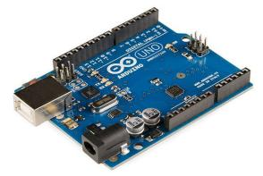
The Arduino Uno R3 is a microcontroller board based on the ATmega328. It has 14 digital input/output pins (of which 6 can be used as PWM outputs), 6 analog inputs, a 16 MHz crystal oscillator, a USB connection, a power jack, an ICSP header, and a reset button. It contains everything needed to support the microcontroller; simply connect it to a computer with a USB cable or power it with a AC-to-DC adapter or battery to get started.
