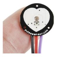
Pulse sensor is designed to give analog output of heart beat when a finger is placed on sensor. It starts working; LED on top side will starts blinking with each heartbeat. To see the sensor output, output pin of sensor is connected to controller. The working principle of sensor is based on light modulation by blood flow through nerves at each heart pulse.
