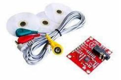
An electrocardiogram (ECG) sensor, also known as an electrical heart rate sensor, is a device that measures the heart's electrical activity and electrical signals in the blood. Cardiologists use ECG sensors to quickly identify abnormal heart rhythms and potential heart disease without intervention. ECG sensors can also help diagnose heart conditions such as coronary heart disease, heart attacks, and angina.
