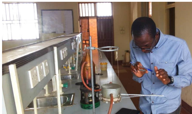
Plate 3: Determination of Cooling Rate using Lee's Disc Apparatus
