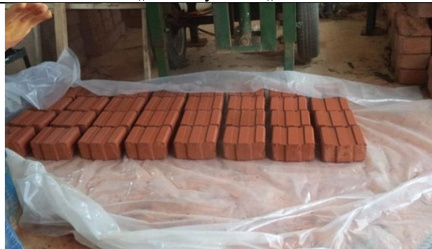
Plate 2: Stacking of NBRRI Blocks for Curing
