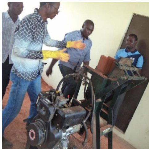
Plate 1: Extrusion of Blocks from the Machine
