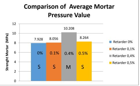
Figure 4. Comparison of average mortar pressure value
