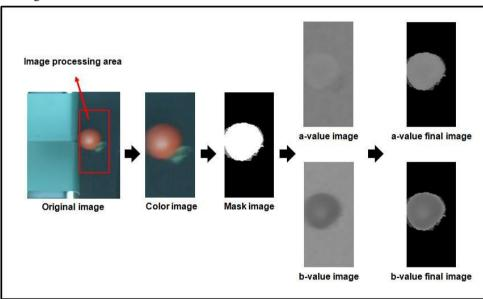
Figure 4: Image processing procedures for tomato
