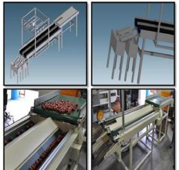
Figure 2: Schematics and photo of the prototype of the color sorting system
