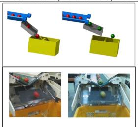
Figure 3: Schematics and photos of the sorting part
