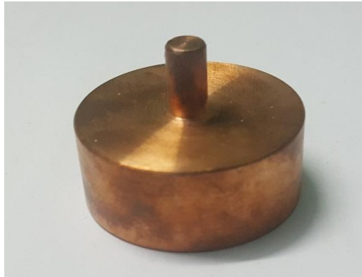
Fig.6 Copper Electrode used for machining
