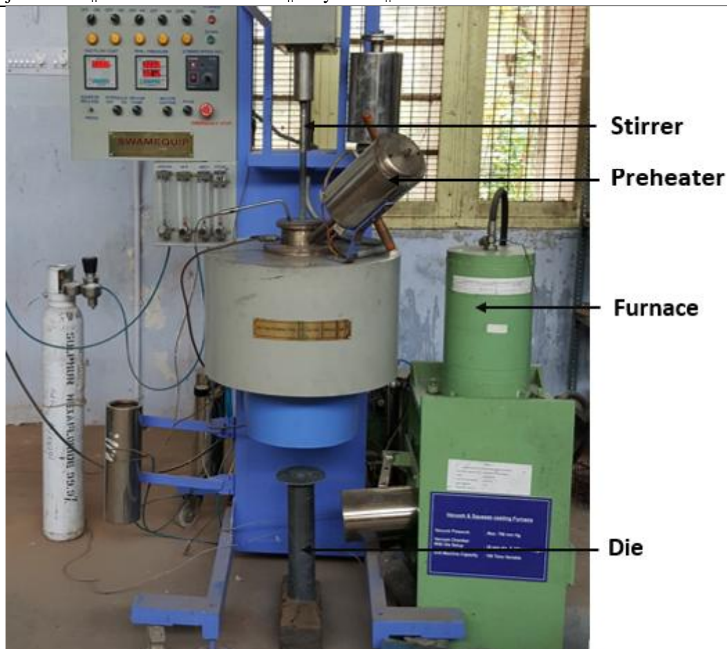
Fig.2 Stir Casting Setup
