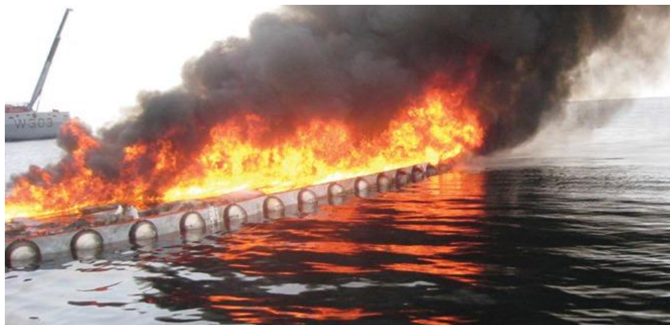
Figure 4. Oil-situ burning method
