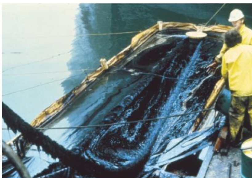
Figure 2. Rope skimmer for recovering the crude oil
