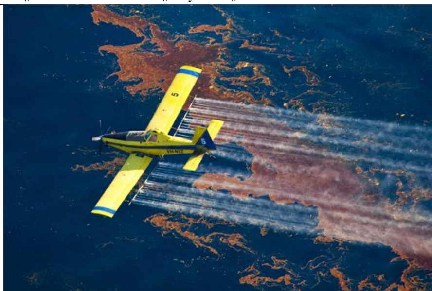
Figure 5. Using dispersant for chemical method
