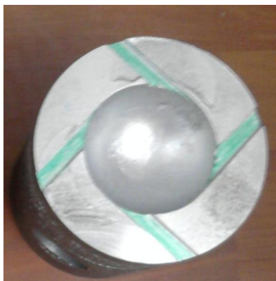
Fig-2 Swirling grooved piston (width 6.5mm depth 2 mm)
