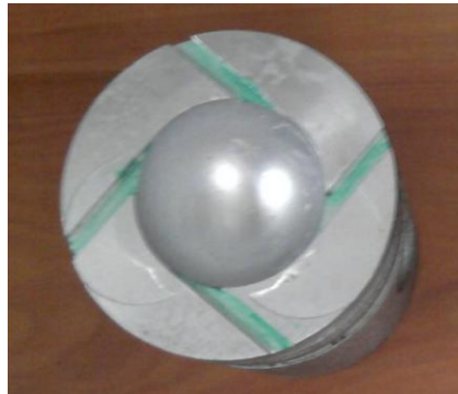
Fig-1 Swirling grooved piston (width 5.5mm depth 2 mm)
