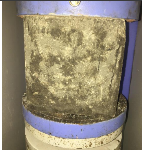
Fig 4: Crack formation of SFRC
